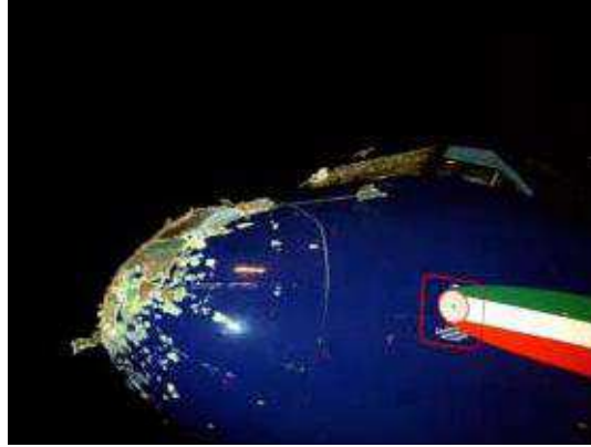
Figure 4.2: Hail can cause major damage to an aircraft
