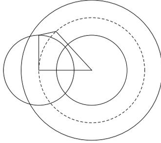
Figure 6: A linkage with four bars with  $l_0 = l_1 = l_3 = 1$  and  $l_2 = 1/2$  together with the work space of the arm of the bars with length  $l_1, l_2, l_3$ .
